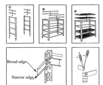
If the connector tabs of the shelf cross pieces should bend on assembly, they can be bent back into their original position with the aid of a flat head screwdriver.
