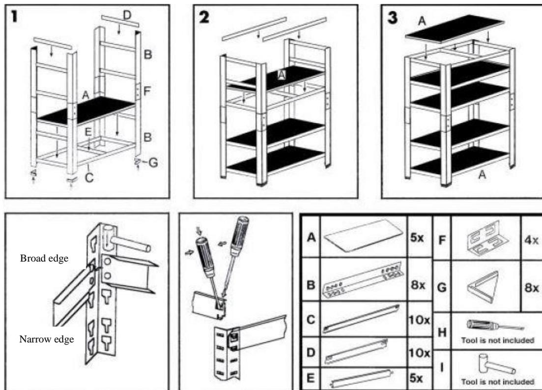
If the connector tabs of the shelf cross pieces should bend on assembly, they can be bent back into their original position with the aid of a flat head screwdriver.
